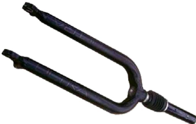
The telescoping tube was made of steel due to the high stress levels on the tube/fork interface resulting in a heavy product. The company had attempted to build an 80mm system from aluminum, but was unable to do so because of the stress at the tube/fork interface.
